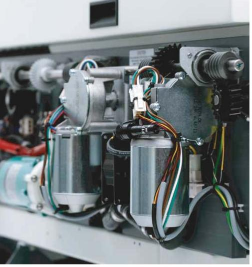
All electrical and me chanical components are located on the sides of the processor, for easy and convenient access during mainentance.
